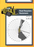
The diagrams represented in this poster show the blind spots for objects at 1500 millimeters from the ground – or the approximate height of a construction worker as observed by the equipment operator. Shorter objects (such as traffic control devices or bent workers) will result in larger blind areas.
